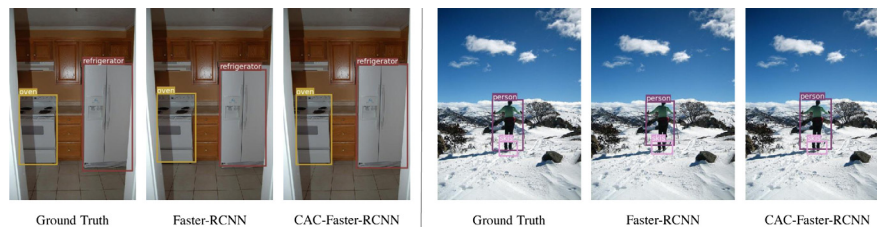
Fig. 7. Visual comparison of different object detection methods. The first column shows the input images with the corresponding ground truth bounding boxes. The second and third columns show the bounding boxes predicted by different models.
